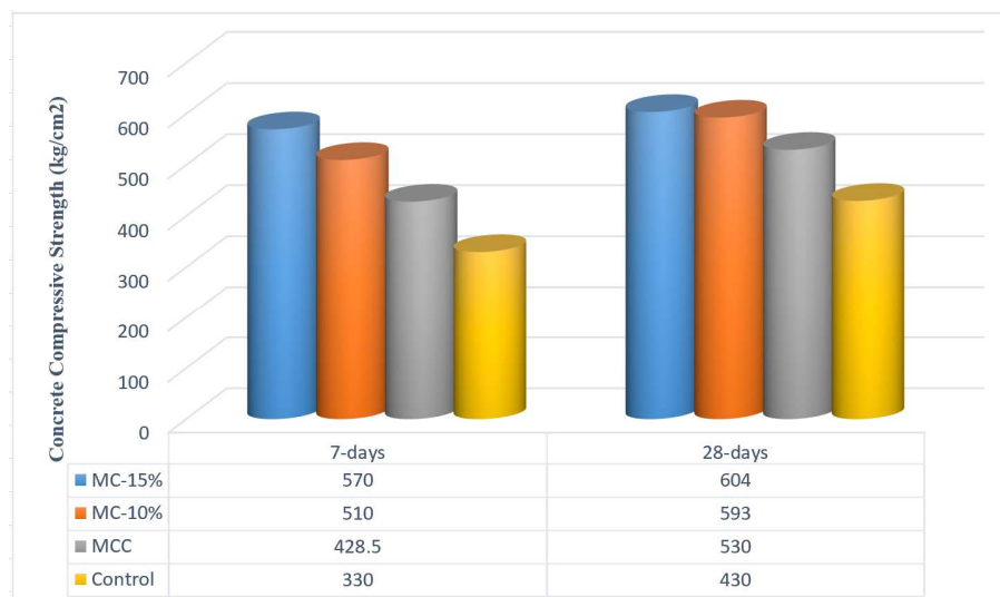
Figure 2. Concrete compressive strength for 7- and 28-days test.
