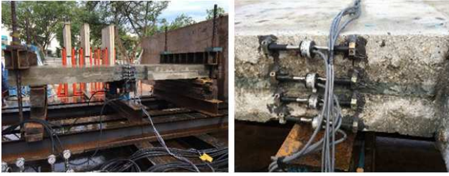
Figure 10. Bending test set-up.
