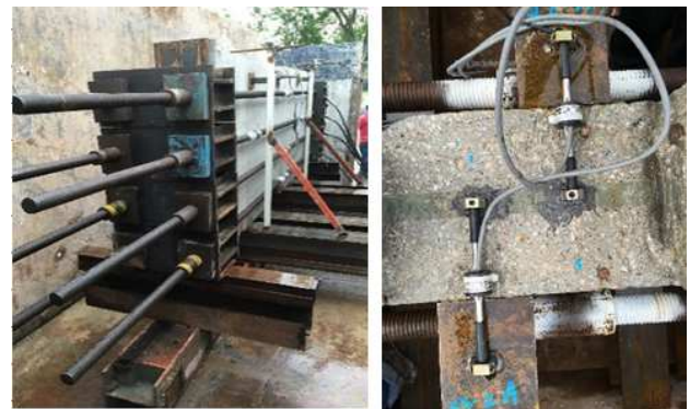
Figure 9. Compression test set-up.
