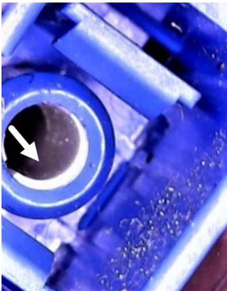
Figure 2. Alignment sleeves are source of potential cross contamination and are not characterized by existing standards.
